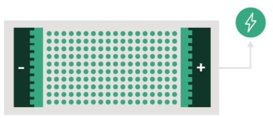
Tabless technology for LiHDX batteries, with low internal resistance
