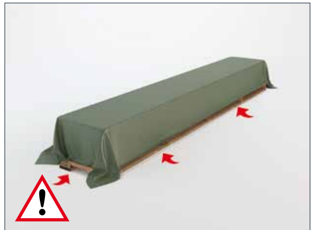
Important: Store materials under a dry and well-ventilated tarpaulin. If the product becomes damp, it should be placed on its vertical edge to allow rapid drying. Never install wet products.
