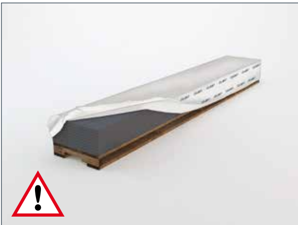
The original packaging may have sustained damage from transportation. Remove the plastic packaging immediately upon delivery at the building site, to avoid risk of efflorescence.
