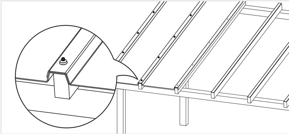
Fix both panels overlap, using specified screws and washers through the pre-drilled holes. Start at the bottom edge and work your way up.
