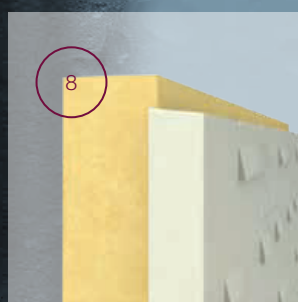
8. Raised insulation at junction acts as a barrier against mortar squeeze.
