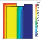
It has been estimated that up to 30% of the heatloss in a well insulated house is through 'Non Repeating Thermal Bridges' at wall/floor junctions, corners, reveals, ceiling junctions heads and sills.
