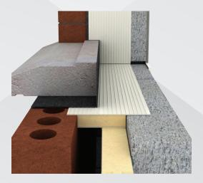
If precise fitting of windows can not be guaranteed, a checked reveal using a vertical DPC should be used.
