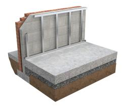
**4.** Lift the insulation board into position using wedges on the floor. Insulation should be cut back to accommodate an adjoining panel at external corners. Joints should be tightly butted.
